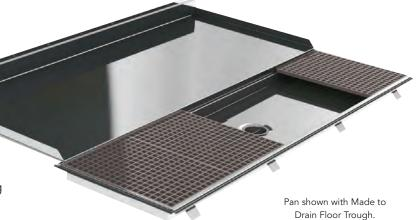
The drain pan is seamless, watertight and 100% sanitary. The pan has a built-in ¼" (6) pitch per foot, which creates a positive pitch to the floor trough and allows drainage of water during equipment operation and cleaning. This pan eliminates free standing water and thoroughly protects against leaks into occupied spaces below the kitchen. The pan is also ideally suited to join together with Made To Drain's full line of floor trough products.
